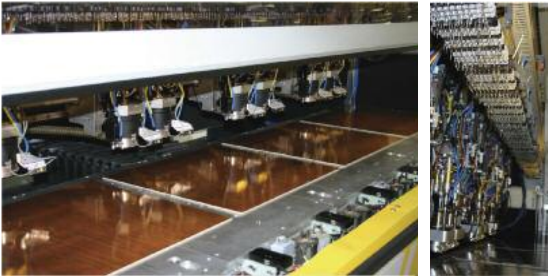
Fig. 9: Drilling of printed circuit boards with cemented carbide drills; drill diameters down to 150 \mu\text{m} ; rotating speed up to 300,000 rpm; cemented carbides which are used for this application must have a high hardness (ultrafine grain) and high modulus of elasticity (660 GPa) for precision drilling of very small holes into a copper/glass-fiber reinforced plastic laminate; courtesy of AT&S.
