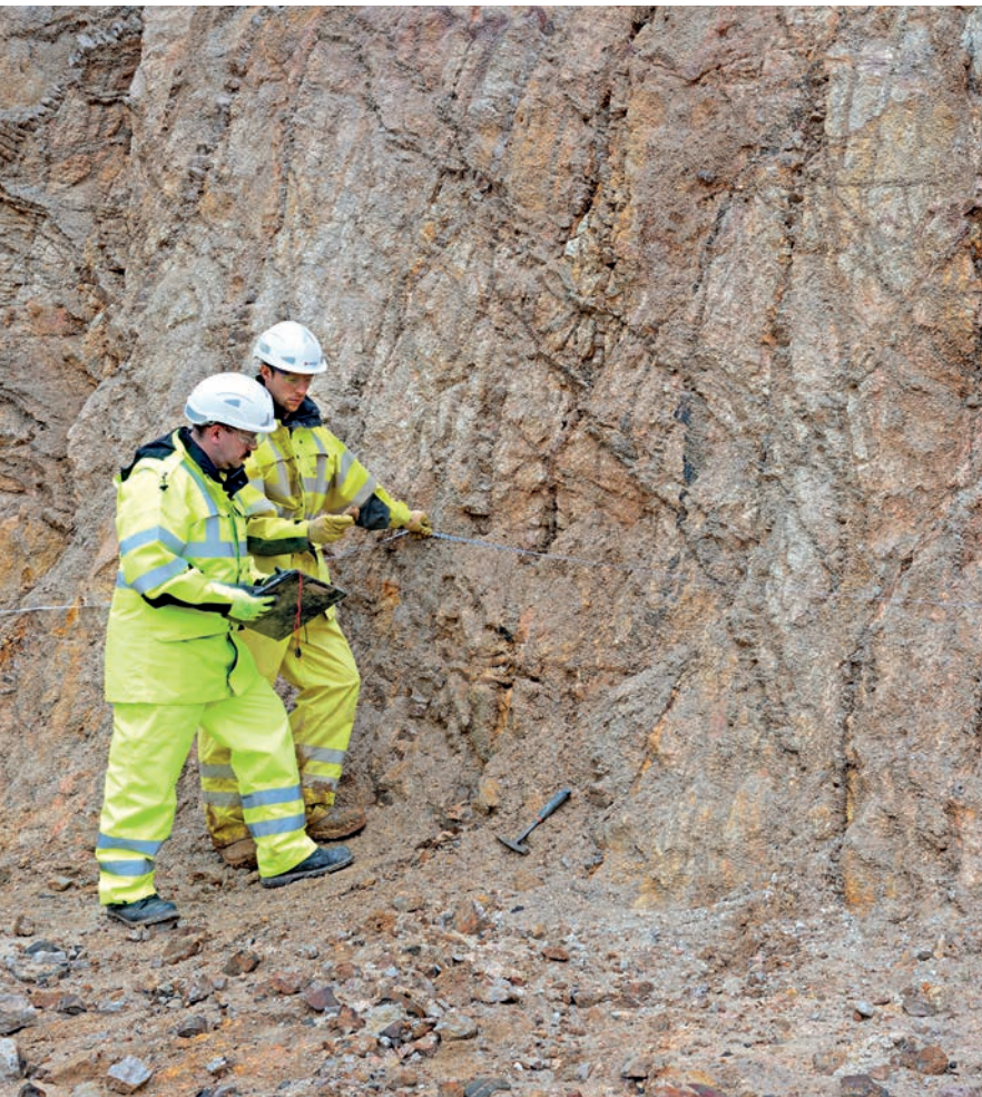
Face showing quartz veins within the granite ore body
