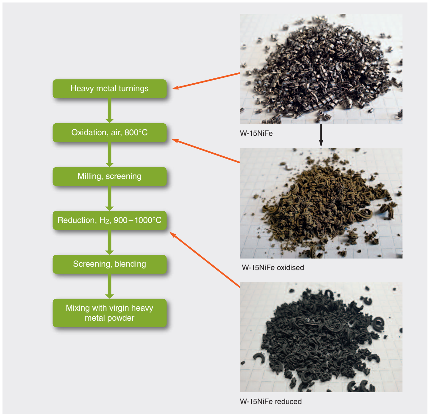
Figure 8: Flow-sheet demonstrating the direct recycling of clean heavy metal turnings by oxidation in air and subsequent hydrogen reduction. Original turnings and the respective oxidised materials are shown in the images to the right hand side. On oxidation different tungstates are formed besides WO 3 which give their colours to the reaction product [(Fe,Ni)WO 4 ]. Contaminated material is pressure digested and tungsten is converted into high purity APT by chemical recycling. Courtesy of Prof. Schubert/TU Wien
