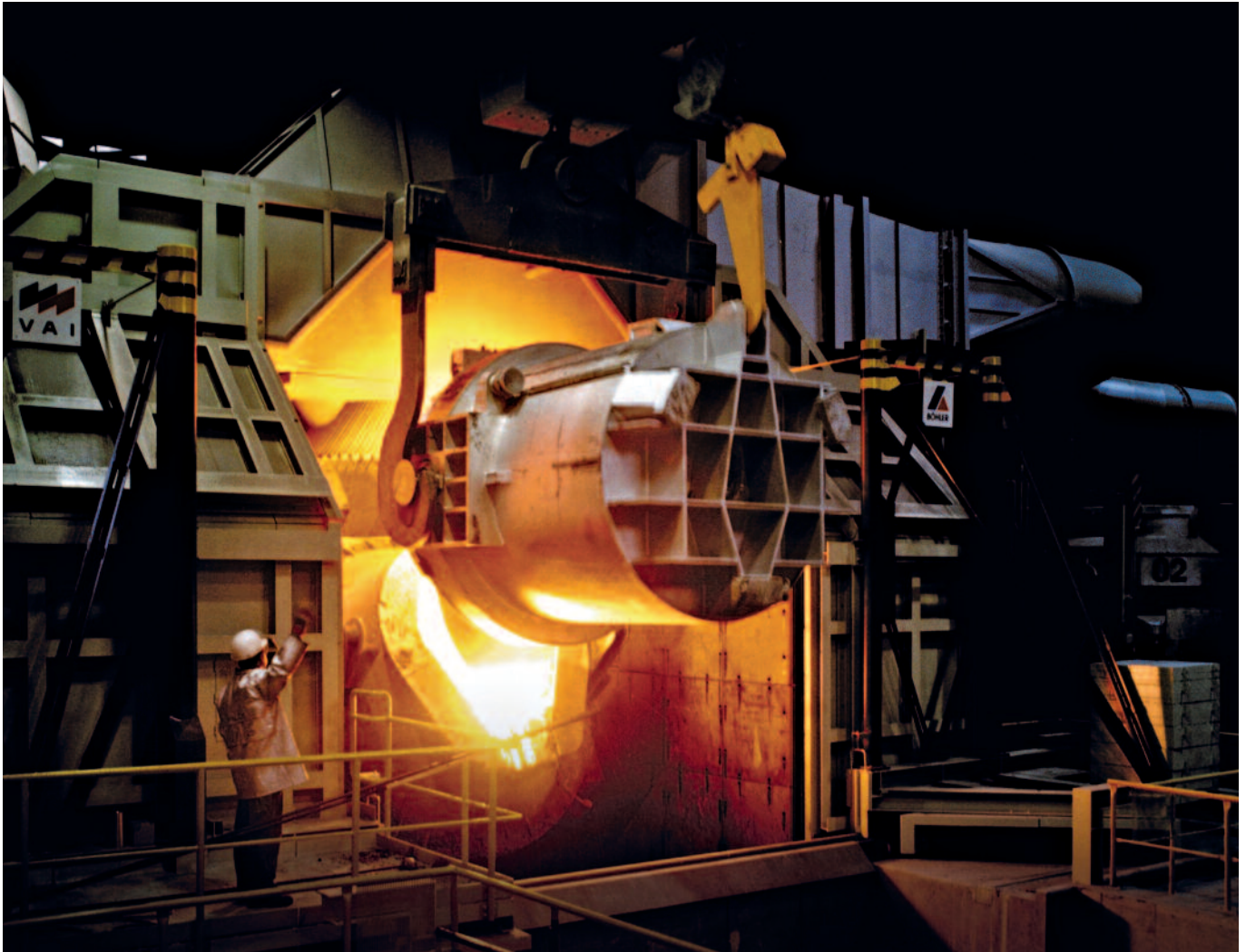
Figure 18: Tungsten recycling in melting metallurgy. Scrap is added to the electric arc furnace (EAF, below) to adjust the desired steel composition (ie for HSS applications). The melt is then transferred to an argon oxygen decarburisation converter (AOD, above) for further refining. Courtesy of GT Engineering, Italy and voestalpine BÖHLER Edelstahl GmbH & Co KG
