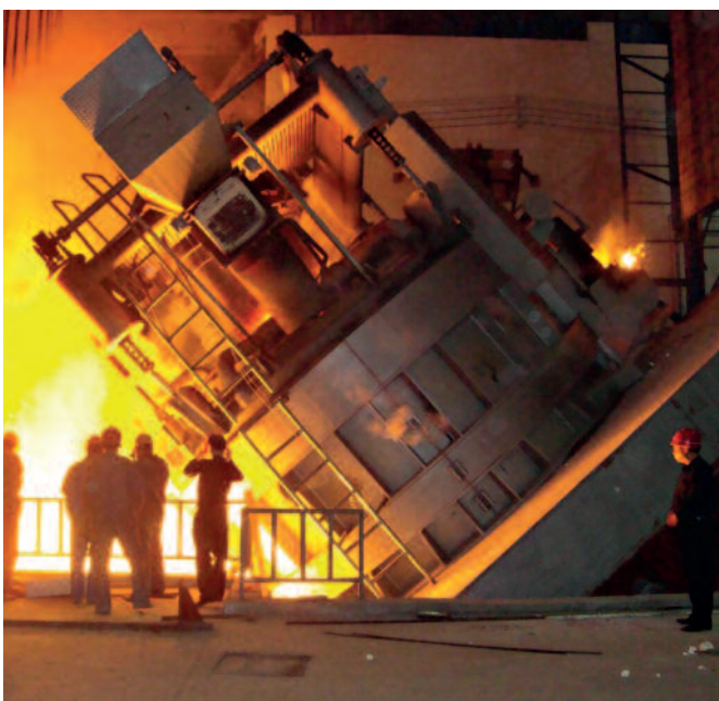
Figure 18: Tungsten recycling in melting metallurgy. Scrap is added to the electric arc furnace (EAF, below) to adjust the desired steel composition (ie for HSS applications). The melt is then transferred to an argon oxygen decarburisation converter (AOD, above) for further refining. Courtesy of GT Engineering, Italy and voestalpine BÖHLER Edelstahl GmbH & Co KG
