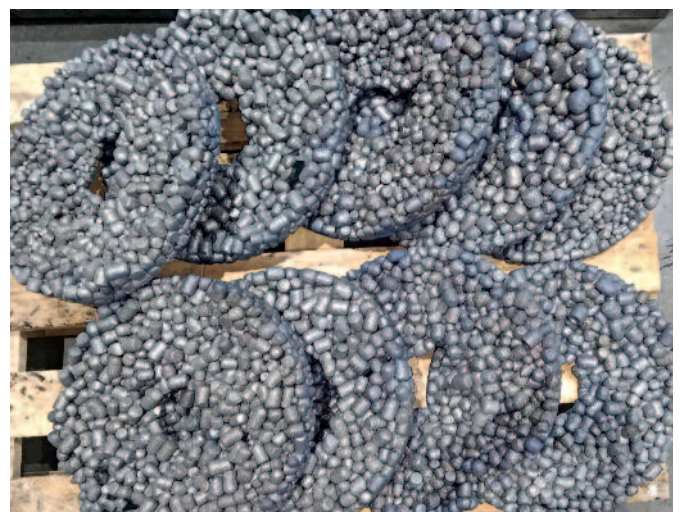
Figure 5: Bloating cemented carbide mining bits. Bloating is done by heating the scrap under hydrogen up to 1900°C. Courtesy of Wolfram Bergbau und Huetten AG
