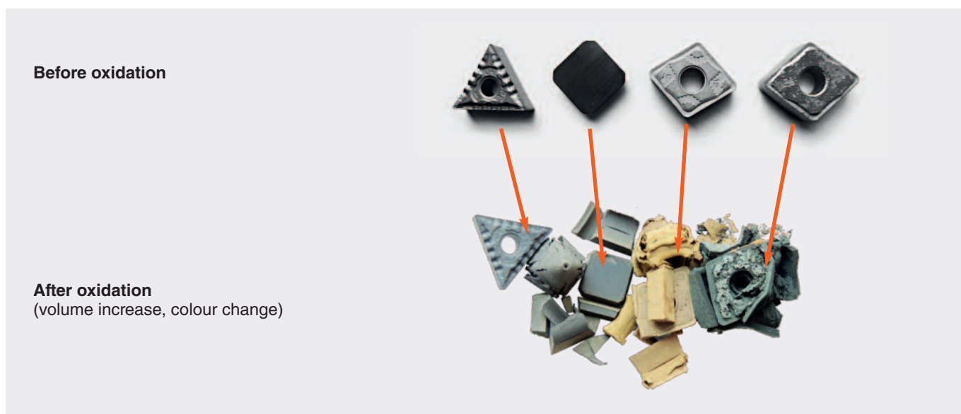
Figure 11: Oxidation of tungsten scrap in air at 900°C. Four different cutting inserts, from left to right: Ti(C,N)-based cermet, WC-Co-Ni grade, WC-Ni-Cr grade and WC-Co grade, before and after oxidation. The cermet (to the left) is not affected and only the surface is slightly oxidised. All other inserts are fully oxidised. The colour of the oxidised insert is a function of the composition (ie third from left: yellow colour of Ni tungstate).
