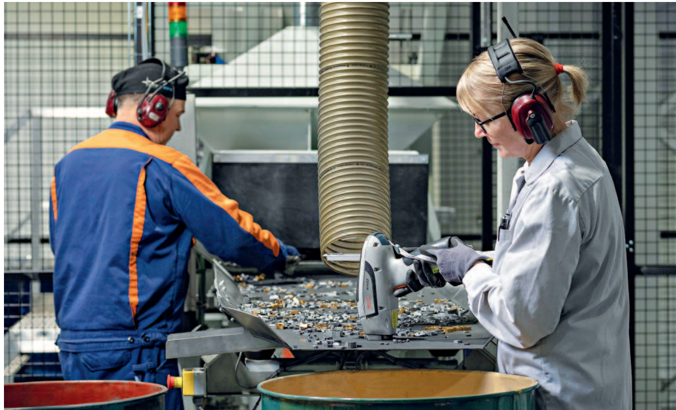
Figure 6: X-ray fluorescence assisted sorting. Sophisticated technology is required to guarantee premium quality reclaim powders. Courtesy of Tikomet Oy
