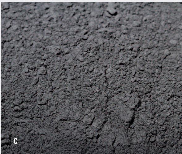
Figure 3: Changes in morphology during the Zn-process. Sorted cemented carbide round tool scrap as input material for Zn-recycling (A). Round tool scrap after reaction with molten zinc and vacuum distillation (B). Final Zn-reclaim powder after ball milling, screening and carbon adjustment, ready to use for RTP (ready-to-press) powder production (C). Courtesy of CERATIZIT S.A.
